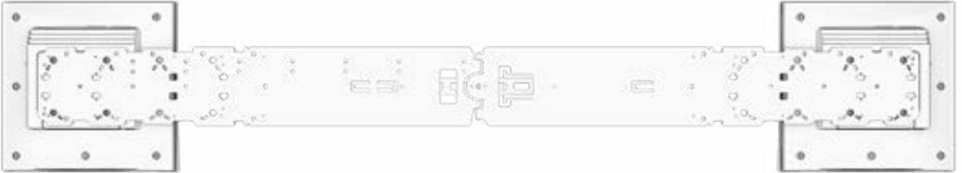
Ensure the **CEILING BRACKET** is level
